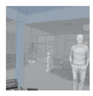
When an sphere or cylinder is first placed into a scene it has a blue tint with a light wireframe over it. This indicates that the object is in edit mode and can be manipulated.
