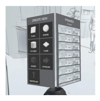
Storyboard VR works in a similar way to traditional storyboard techniques by creating static frames that roughly block in a scene. Scene frames are accessed via the Frames directory by rotating the left hand controller. The frames directory shows a thumbnail of each frame within the flow.
