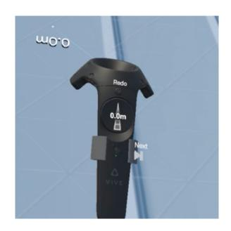
To scale the floor, *slide up or down on the right controller thumbpad.*The floor size appears alongside
